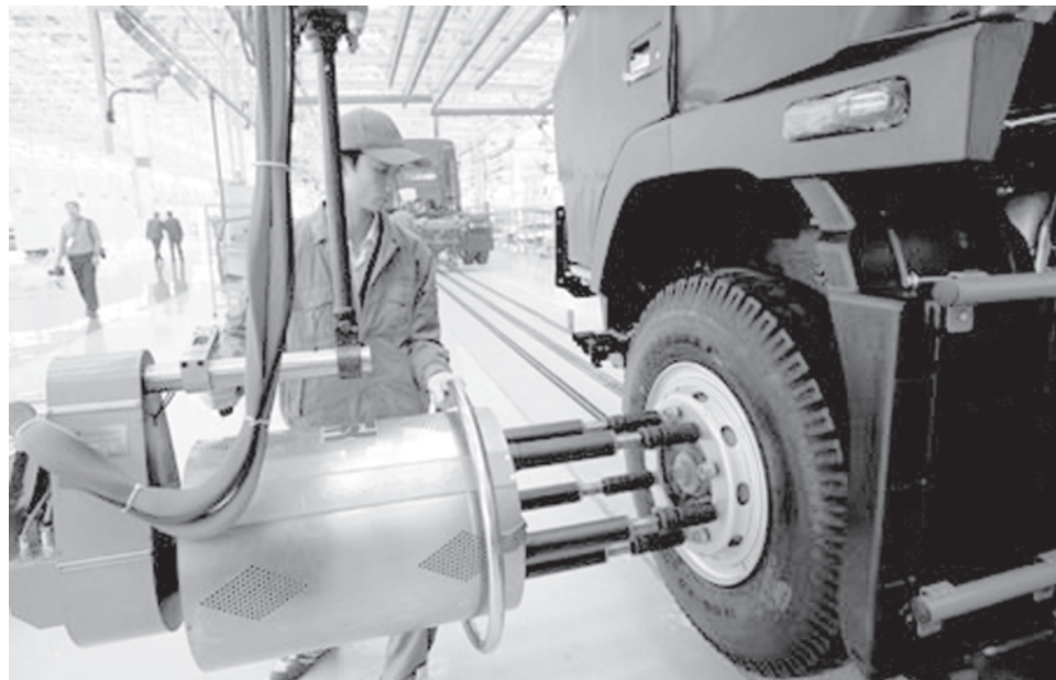
A worker is busy with fitting in the wheel hub, on the heavy truck production line of the Shanxi Dayun Automobile Production Co Ltd, as the ceremony marking the formal production of Dayun Heavy-Duty Trucks is held here, in Yuncheng City, north China's Shanxi Province, on 26 Oct, 2009. —XINHUA
