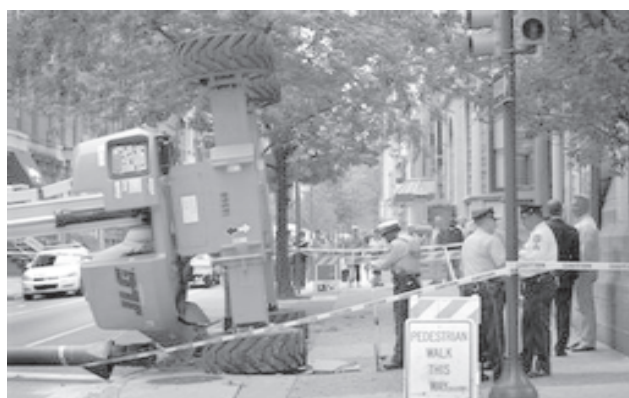
Police and fire department officials gather at the accident scene in centre city Philadelphia on 12 Oct, 2009, where a man operating a construction lift to work on a church roof drove over a sidewalk grate, slowly toppling the crane-like machine and sending him 125 feet to the ground.—INTERNET
