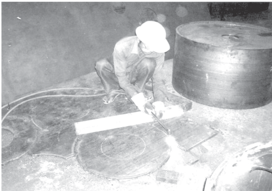
A labourer works in a workshop to make rollers for road-rollers.
