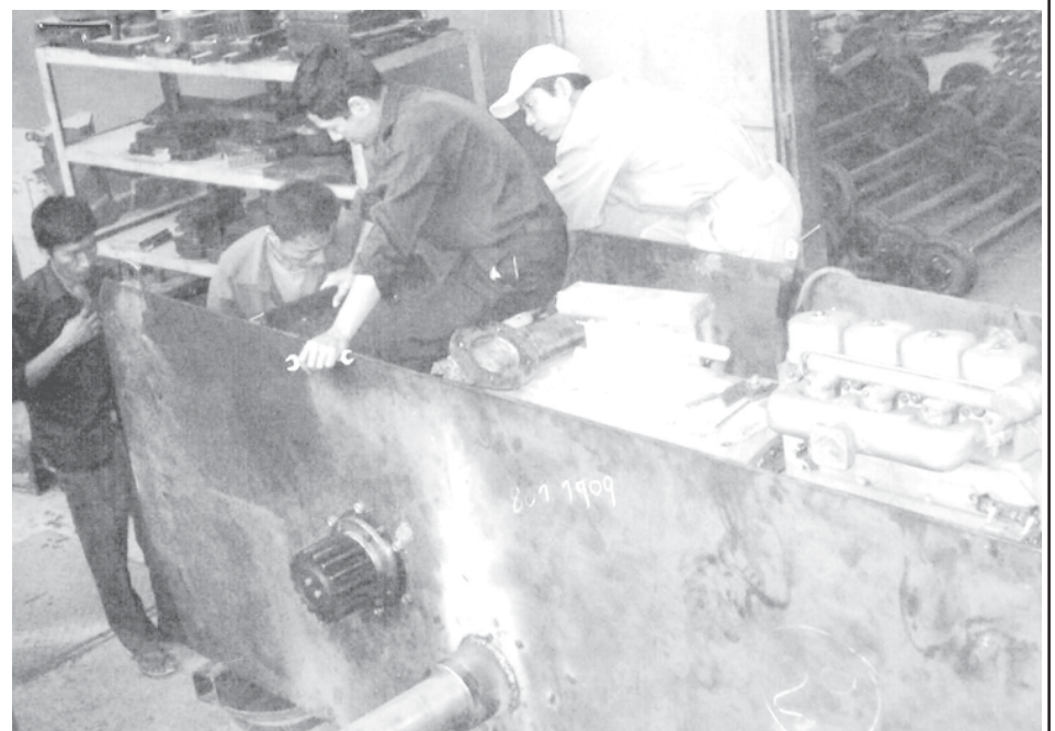
Workers assemble body of a road-roller.
