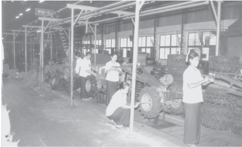
Workers assembling Ayeya-1 power-tillers.
