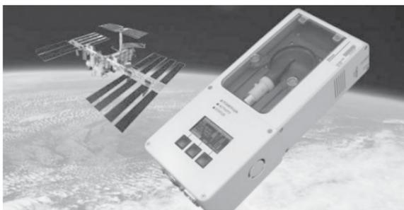
The ENose flew for six months on the International Space Station monitoring the air the astronauts breathed.
