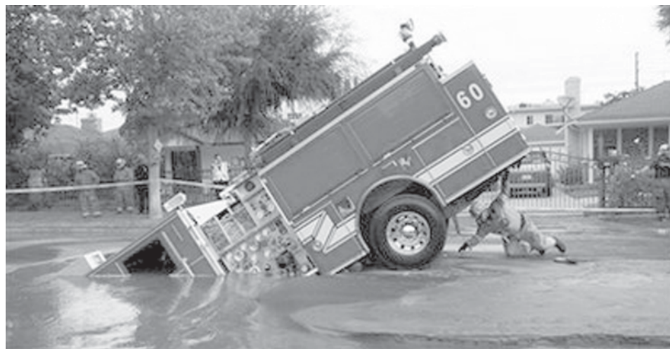
A Los Angeles fireman looks under a fire truck stuck in a sinkhole in the Valley Village neighbourhood of Los Angeles on 8 Sept, 2009. Four firefighters escaped injury early Tuesday after their fire engine sunk into a large hole caused by a burst water main in the San Fernando Valley, authorities said.—INTERNET
