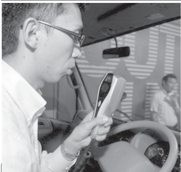
A Toyota Motors engineer blows into a hand-held breathalyser and camera unit during a press preview by Toyota Motors on their breath-alcoholignition-interlock system in Tokyo, on 31 August. Toyota said on Monday it was developing the anti-drunk driving equipment that would lock the ignition of a vehicle if high levels of alcohol are detected in the driver.—INTERNET
