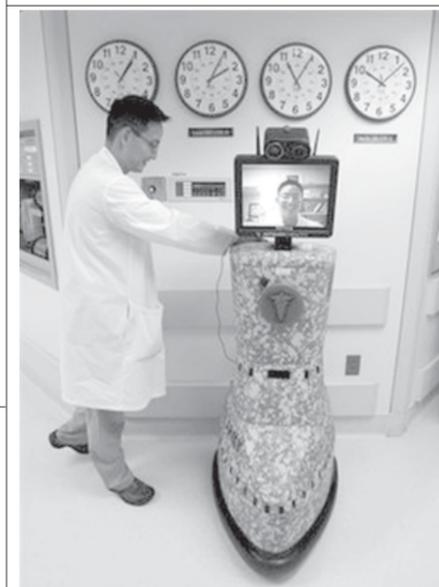
In this 17 Aug, 2009 photo, Dr Kevin Chung moves a medical robot, nicknamed the 'Chungbot,' into position to be re-charged, at Brooke Army Medical Center in San Antonio. The robot is controlled with a laptop and joystick and wirelessly transmits images and sound between the user and the patient, allowing for follow-up from around the world or quick diagnosis from a far-off specialist.
