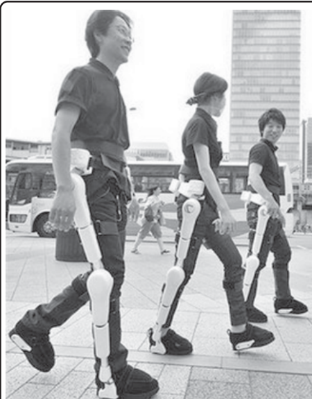
Japan's robotics venture Cyberdyne employee wearing the robot-suit "HAL" (Hybrid Assistive Limb) walk on a street in Tokyo for the demonstration. Two men and a woman, wearing what looked like white plastic exoskeletons over black outfits, were testing — at a pace of 1.8 kilometres (1.1 miles) an hour — robotic suits designed to give mobility to the injured and disabled. Japan's robotics venture Cyberdyne employee wearing the robot-suit "HAL" (Hybrid Assistive Limb) walk on a street in Tokyo for the demonstration. Two men and a woman, wearing what looked like white plastic exoskeletons over black outfits, were testing — at a pace of 1.8 kilometres (1.1 miles) an hour — robotic suits designed to give mobility to the injured and disabled.
