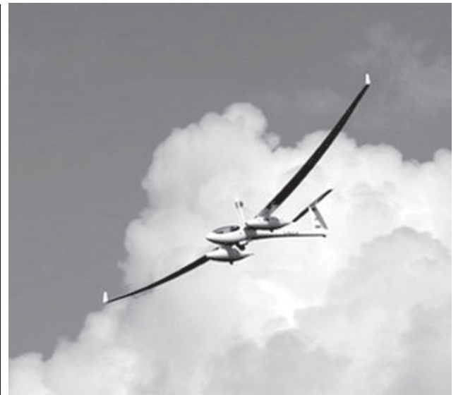
The Antares DLR-H2 flies its maiden voyage over the northern German city of Hamburg. The airplane powered by fuel cells was commissioned by the German Aerospace Centre (DLR) with the goal of developing fuel cells for a reliable on-board power supply for wide-body airliners.
