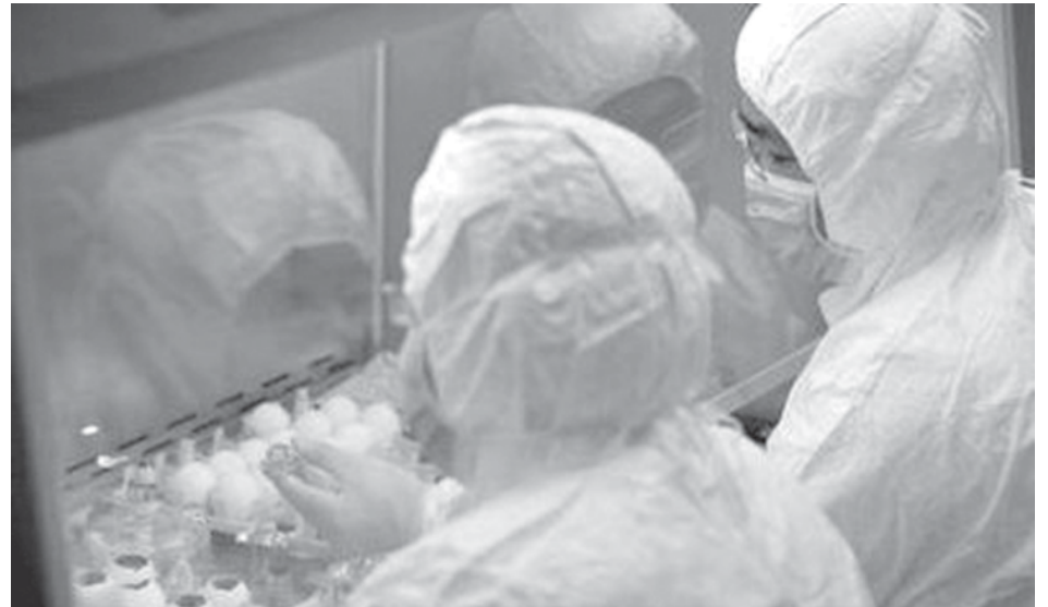
Technicians work with eggs in the inoculation area of Sinovac Biotech Ltd, a Chinese vaccine making company, during production of a vaccine for the H1N1 flu virus in Beijing on 14 June, 2009. Vaccine makers germinate the virus in fertilized chicken eggs in a process that can take four to six months.—INTERNET
