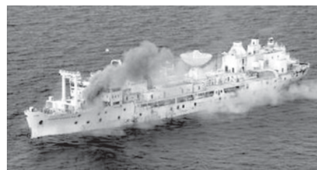
The former US Air Force missile-tracking ship General Hoyt S Vandenberg begins to sink after cutting charges were detonated seven miles off Key West, Florida, on 27 May, 2009. The 523-foot-long Vandenberg was sunk to create an artificial reef to attract recreational divers and anglers. Some 70 percent of the $8.6 million budget was expended to rid the vessel of contaminants before it was scuttled.
