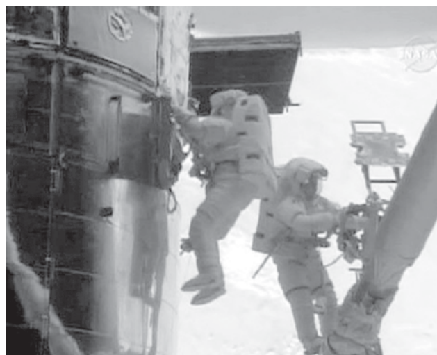
Astronaut Andrew Feustel (L) and John Grunsfeld, on Atlantis’ robot arm, work on the Hubble Space Telescope with the coast of Africa in the background in this image from NASA TV on 18 May, 2009. Shuttle Atlantis astronauts returned to the Hubble Space Telescope on Monday for a final spacewalk to install fresh batteries, thermal shields and a sensor to pinpoint celestial targets for research. Grunsfeld and Feustel left the shuttle’s air lock at about 8:30 am EDT (1230 GMT), almost an hour ahead of schedule.—INTERNET
