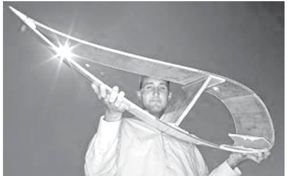
Purdue doctoral student Jonathan White holds a cross section of a wind turbine blade like the one used in research to improve the efficiency of turbines and prevent damage to blades from high winds.—INTERNET
