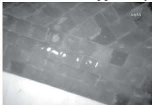
Damage, seen as white marks, along an area of about 21 inches (53 cm) spanning four of space shuttle Atlantis' thermal tiles located on the starboard side of the spacecraft can be seen in this image from NASA TV, on 12 May, 2009.—INTERNET
