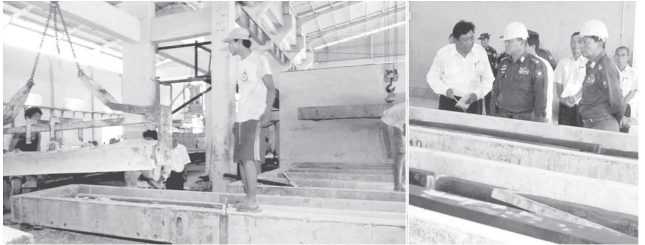
Lt-Gen Khin Zaw inspects production of RC sleepers at RC sleeper factory under the Ministry of Rail Transportation in Mottama.—MNA
