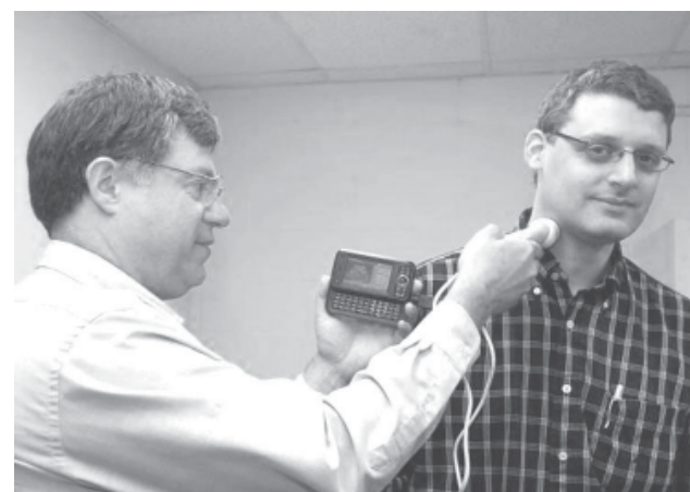
William D. Richard (left) takes an ultrasound probe of colleague David Zar’s carotid artery with a low-power imaging device he designed.
