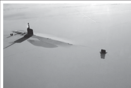
In this photo released by the US Navy, the Los Angeles-class submarine USS Annapolis is seen on the surface of the Arctic Ocean after breaking through three feet (ninety centimeters) of ice during Ice Exercise 2009, a training and research exercise.
