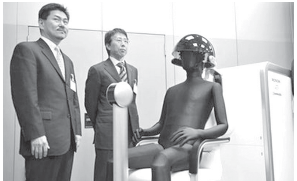
Honda Research Institute president Yasuhisa Arai (L) and Mitsuo Kawato, Japan's ATR computational Neuroscience Laboratories director, stand next to a brain-machine interface, equipped with special headgear to measure slight electrical current and blood flow change occurring in the brain, at Japanese auto giant Honda's headquarters in Tokyo.
