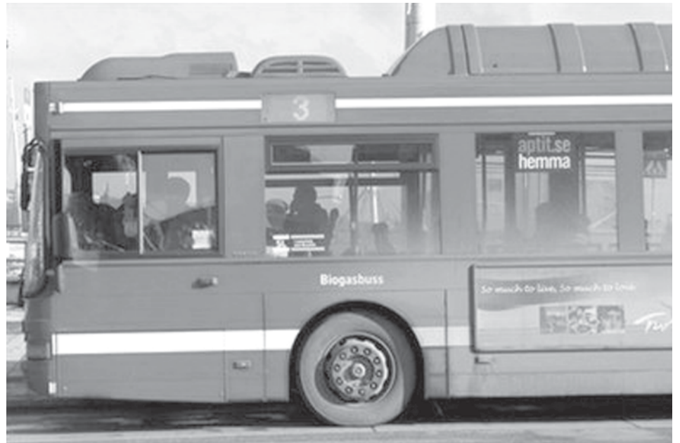
A biogas bus. The city officials of Oslo plan to introduce as of 2010 buses that run on biofuels extracted from wastewater, a "clean" energy consisting of methane generated by fermenting sludge.—INTERNET
