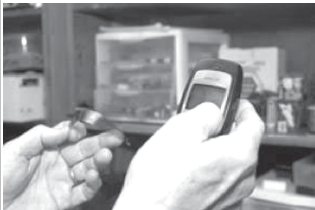
Mast created a new antenna using a spun carbon nanotube thread and sticky tape.
