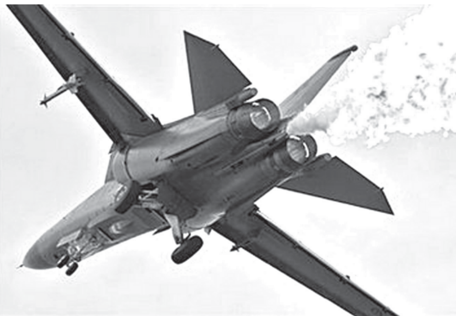
Burning fuel : A Royal Australian Airforce F111 performs a fuel dump and burn at the Australian International Airshow near Melbourne.
