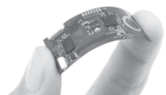
IMEC's flexible wireless monitoring system for vital body parameters with embedded microcontroller chip.
