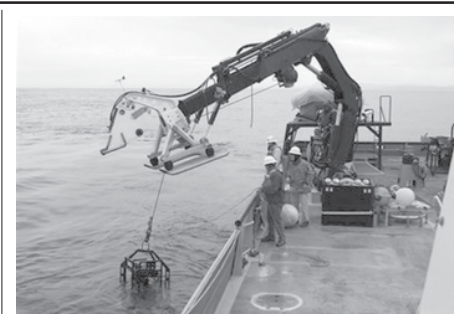
The 502-pound deep sea video camera 'Eye-in-the-Sea' aboard the Research Vessel Point Lobos , is lowered into the Pacific Ocean 22 miles off the California coast. The Eye-in-the-Sea is the world's first Web camera that will offer a window into the darkness of the deep ocean.
