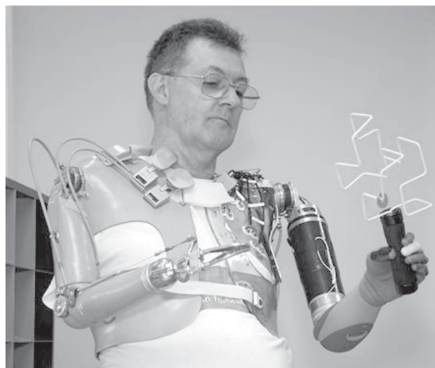
Jesse Sullivan, 61, from Dayton, TN, demonstrates advanced, multi-degree control of the JHUAPL Proto 1 arm at the Rehabilitation Institute of Chicago. Sullivan, who lost his arms in an electrical accident in 2001, was the first person to receive the targeted muscle reinnervation (TMR) procedure in 2001.—INTERNET
