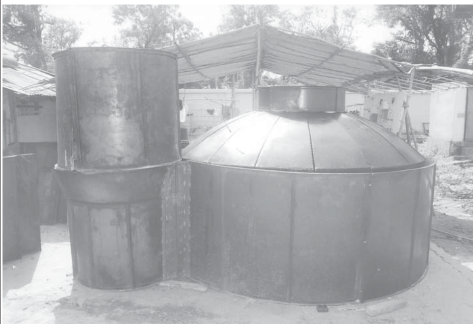
Steel biogas digester to be kept inside a biogas unit.
