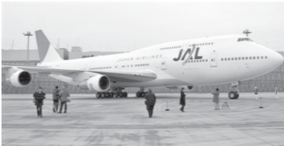
Biofuel-loaded Japan Airlines Boeing 747-300 sits on the ground during the demonstration of its engine ground-run test at Tokyo International Airport in Tokyo, on 29 Jan, 2009. Using blend of 50 percent biofuel and 50 percent traditional Jet-A jet (kerosene) fuel, JAL conducts an hour-long demonstration flight on Friday.—INTERNET
