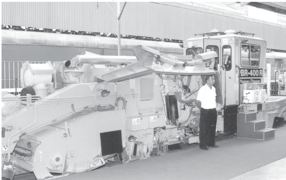
Indian-made profile ballast regulator.
