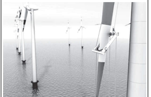
A robot inspects a wind energy converter's rotor blades for possible damage.
