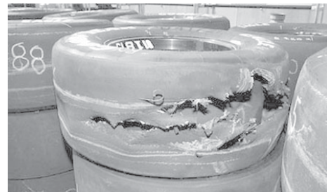
A damaged right rear tire sits in the garage area during the NASCAR Allstate 400 at the Brickyard auto race at Indianapolis Motor Speedway in Indianapolis, on 27 July, 2008. Teams experienced unusual tire wear in the race.—INTERNET
