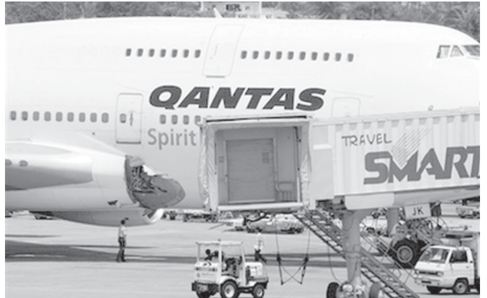
An airline mechanic looks at the damaged right wing fuselage of a Qantas Airways Boeing 747-400 passenger plane following an emergency landing at the Ninoy Aquino International Airport on 25 July, 2008 in Manila, Philippines. The plane, with 350 passengers and 19 crew, was enroute to Australia from London when a loud bang punched a hole in the right wing fuselage, passengers said.—INTERNET
