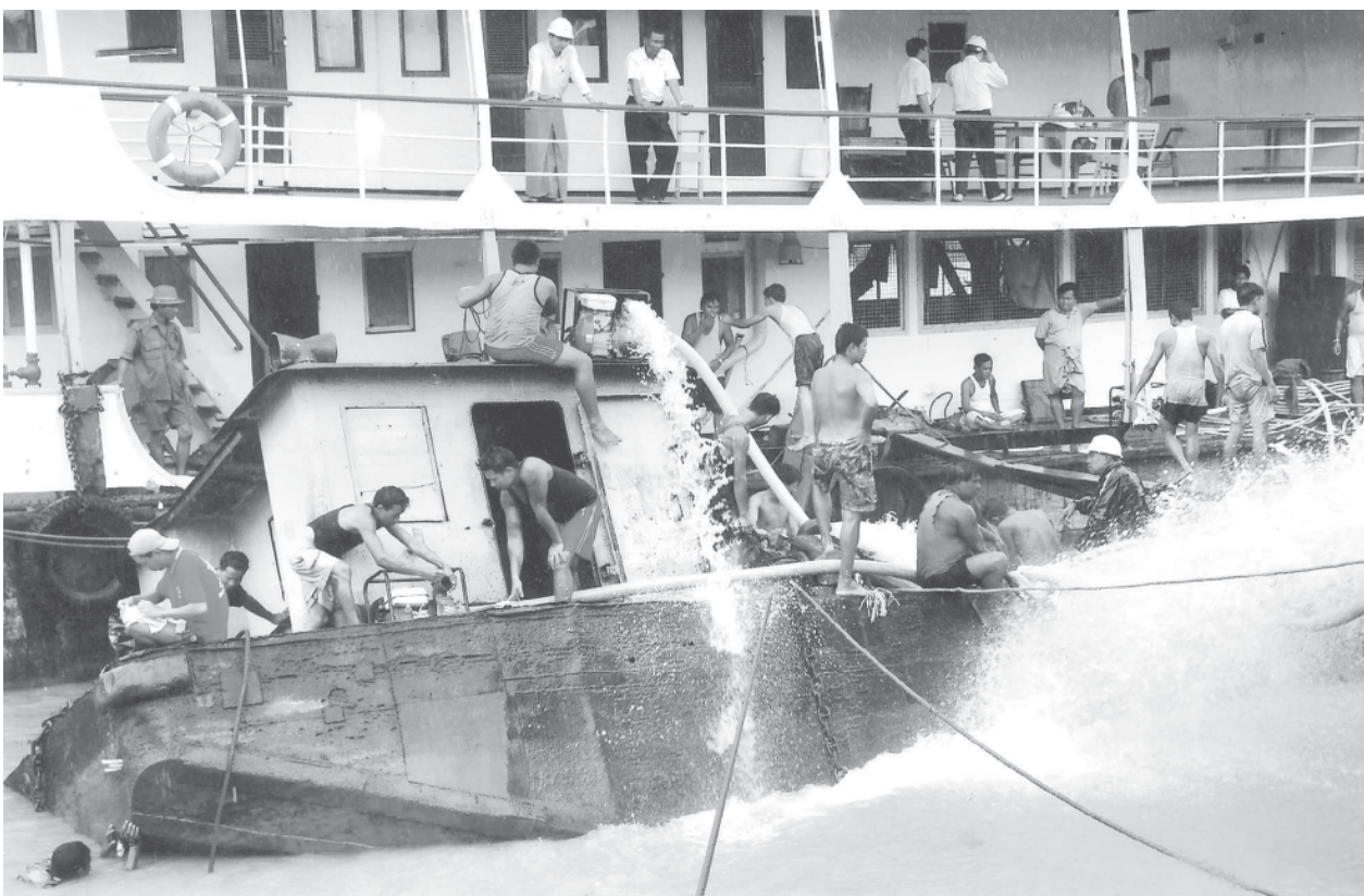
Workers salvaging a sunken pontoon at Mawlamyinegyun Port.
