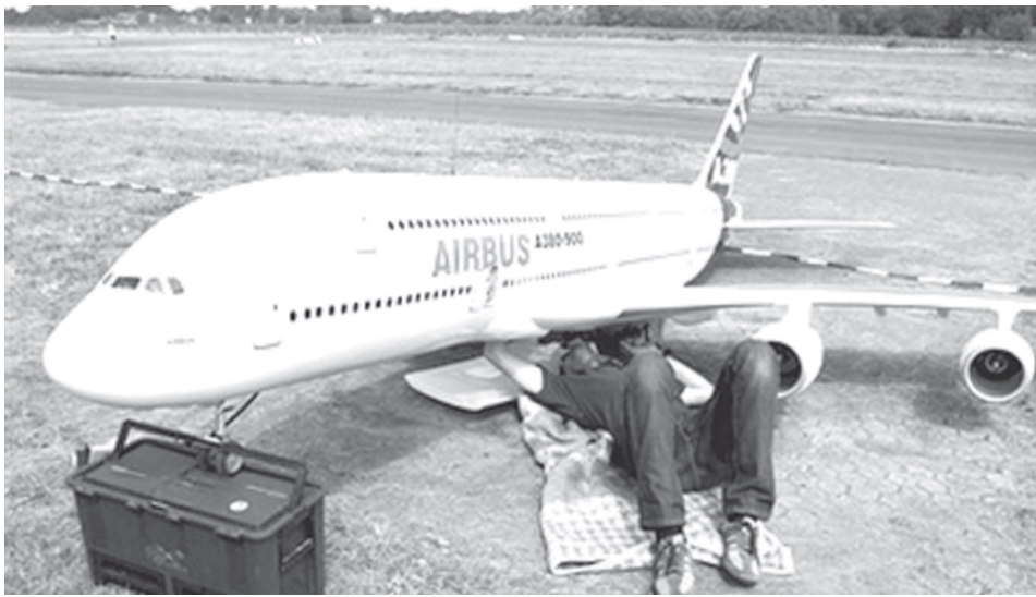
Model maker Reinhard Oetken prepares his Airbus 380-900 model aircraft for a flight during a model jet meeting at the airbase Ganderkesee, northern Germany, on 6 July, 2007. The airplane is 5.25 meters (17.24 feet) long, wing span is 5.35 meters (17.55 feet) and it weighs 97.5 kilogram. Its tank is filled with 21 liters of kerosene. Germany's largest model aircraft flew the first time in public on Sunday . — INTERNET
