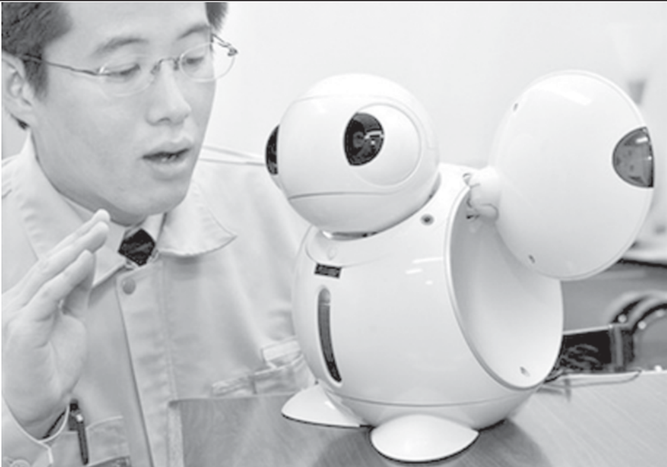
Researcher for Japanese electronics giant Toshiba, Daisuke Yamamoto, displays the prototype model for the new desktop-sized robot called the “ApriPoco”, which can recognize human voices and operate electronic devices such as televisions and air conditioners, at the company’s laboratory in Kawasaki, Japan.—INTERNET
