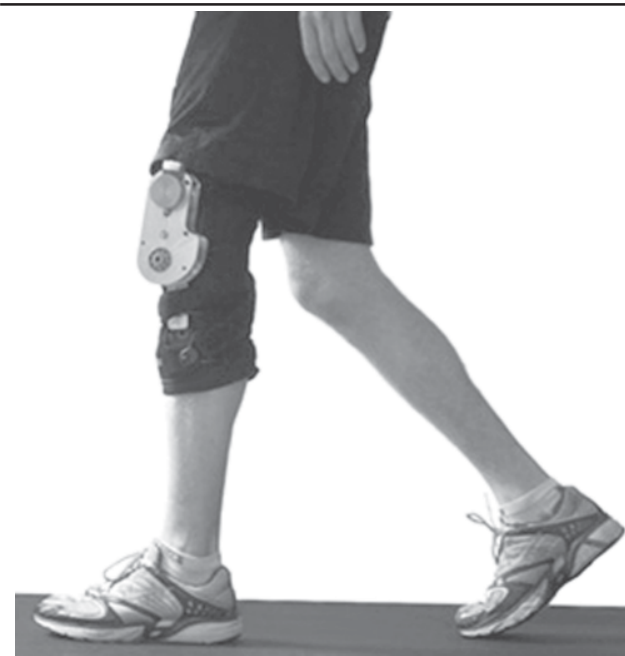
A new energy-capturing knee brace can generate enough electricity from walking to operate a portable GPS locator, a cell phone, a motorized prosthetic joint or an implanted neurotransmitter, research involving the University of Michigan shows.—INTERNET
