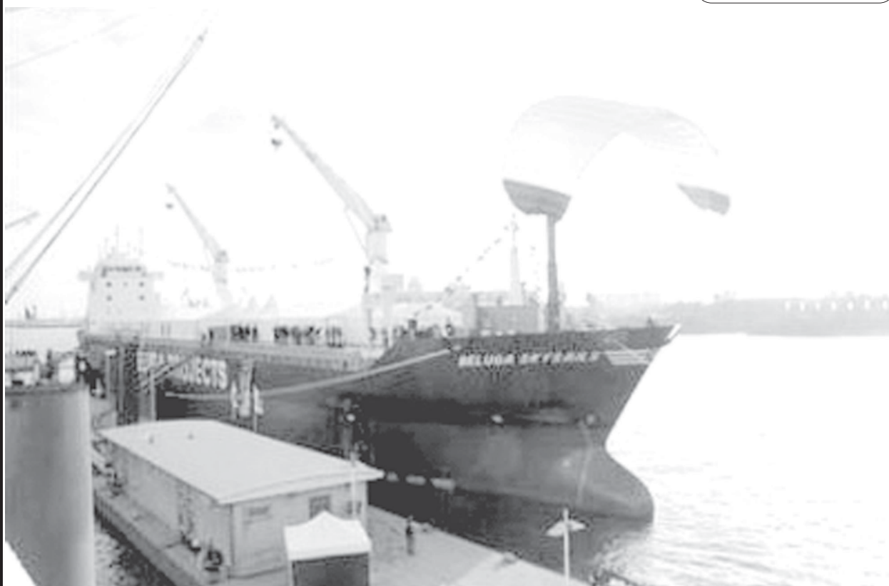
A tanker, pulled by a SkySails high-tech kite, the world's first commercial ship pulled by a high-tech kite designed to cut fuel consumption and reduce greenhouse gas emissions sets off on its eagerly awaited maiden voyage from Germany on Tuesday. — INTERNET
