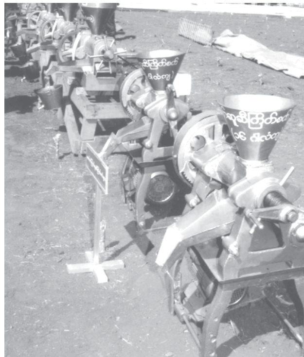
Sixteen-gallon capacity jatropha curcas seed milling machines produced by Shan State (North) Peace and Development Council.
