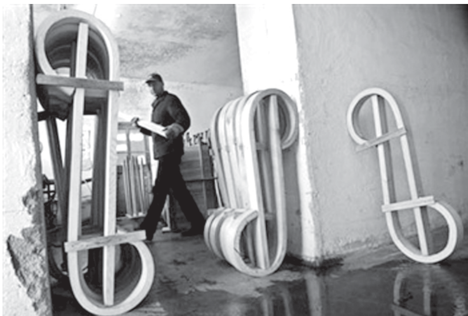
Manfred Wassermann, employee of a traditional wooden sledge manufacturer, checks the curved ash wood in Boehen, about 120km (75miles) south of Munich, on 7 Nov, 2006. Bavarian company Sirch Wood Processing produces more than 50,000 hand-crafted wooden sledges yearly. —INTERNET
