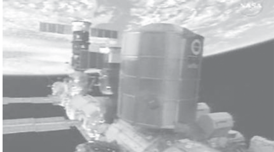
The Leonardo multi-purpose logistics module is seen docked to the Unity node of the International Space Station with the earth in the background, in this view from NASA TV on 13 July, 2006.—INTERNET
