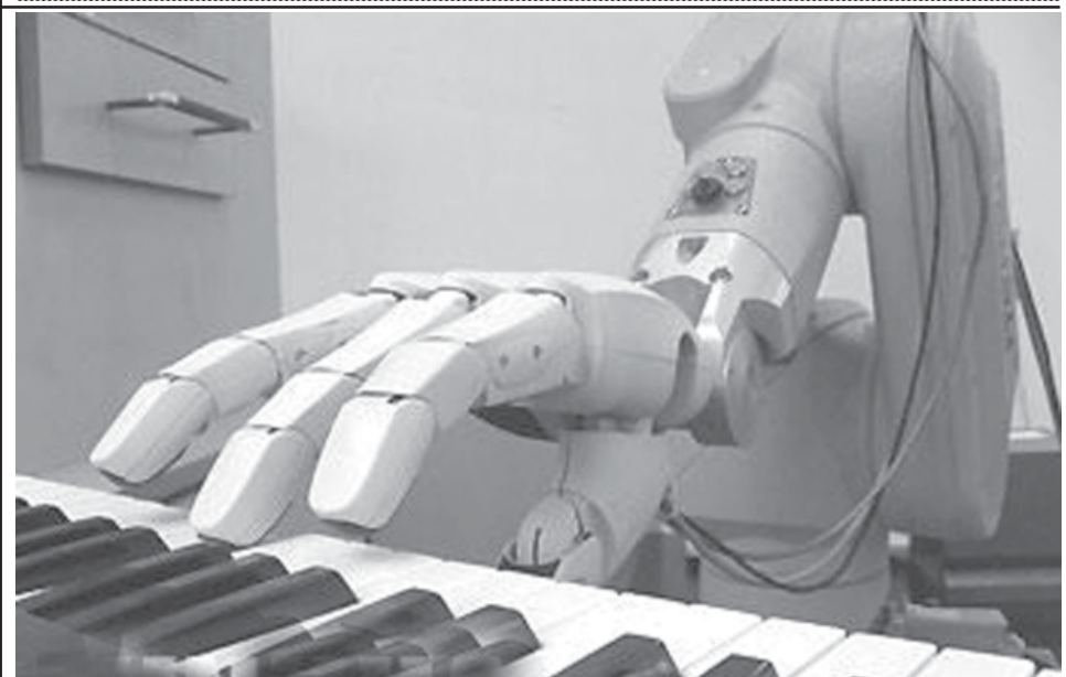
A robot hand performs electronic organ by instructions in Harbin, northeast China's Heilongjiang Province, on 26 June, 2006. The four-finger robot hand was co-devised by Harbin Institute of Technology and German Aerospace Centre, which consists of thirteen movable parts and can accomplish multiple sense-and-action functions.—INTERNET
