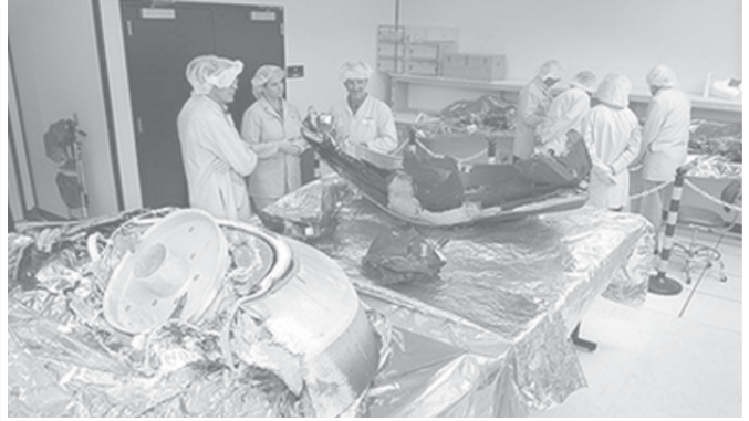
In this photo released by NASA, large sections of the Genesis space probe that survived the hard-impact landing in the Utah desert on 8 Sept, 2004, are examined by scientist at Lockheed Martin's facilities on 24 Sept, 2004, in Denver. NASA releases a final report, on Tuesday, 13 June, 2006, on what caused the Genesis space probe to slam into the Utah desert.—INTERNET
