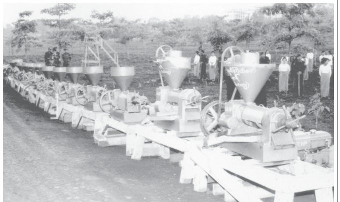
Shan State (North) produces small-scale milling machines to mill physic nut seeds to extract physic nut oil.
