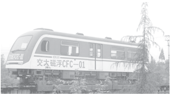
China successfully tested a low-to medium-speed magnetic levitation train, the first domestically developed one in the country, in Chengdu, capital city of Southwest China's Sichuan Province, on 30 April, 2006. The test maglev train is 11.2 meters long, 2.6 meters wide and 3.3 meters high. It ran steadily on a 425-meter-long experimental line. With a weight of 18 tons, the test train can hold 60 people. It can travel at speeds of up to 160 kilometers per hour. INTERNET
