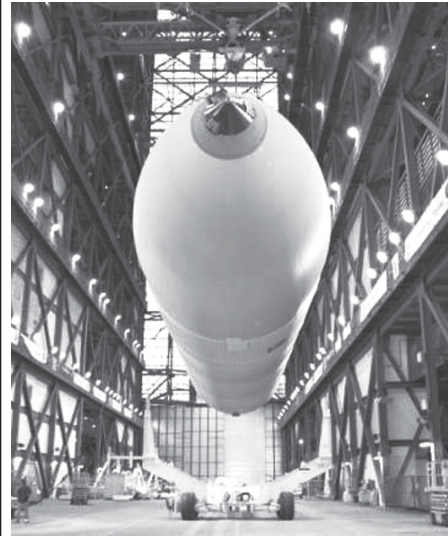
Space Shuttle External Tank 118 (ET-118) is slowly moved above the transporter in the transfer aisle of the Vehicle Assembly Building before being lowered at the Kennedy Space Center, Florida, in this 14 Oct, 2004 file photo. NASA plans to fly the space shuttle Discovery in July without further changes to the external fuel tank, despite some engineers' concerns that the tank needs more work, officials said on 28 April, 2006.—INTERNET
