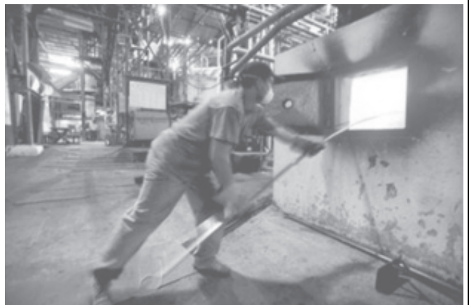
A worker stokes the fire of one of the three-storey ovens that burn cane fibre, generating all the electricity used by the Palo Gordo refinery in San Antonio Suchitepequez, Guatemala on 10 March, 2006. —INTERNET
