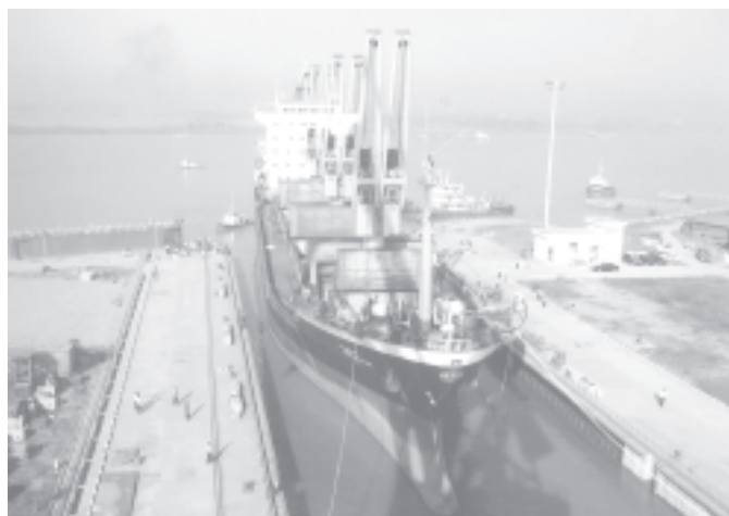
Multi-purpose MV Mandalay of Myanma Five Star Line being docked at 12,000-ton-capacity Dry Dock. — TRANSPORT
