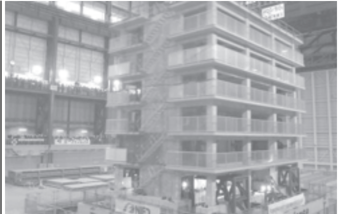
A 16-metre (52.5-foot), 6-storey building is jolted at velocities similar to those in the 7.2-magnitude quake in an experiment in Miki, western Japan, on 13 Jan, 2006. Japanese researchers tested the world's biggest quake simulator 'E-Defence' in a project that could help improve earthquake resistant construction methods.—INTERNET
