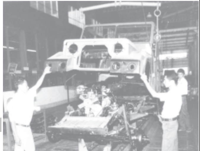
Industry-2 Ministry-made Mazda jeeps being assembled.
