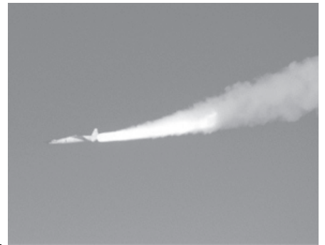
An X-43A scramjet accelerates after it is released from a launch aircraft over the Pacific Ocean. NASA confirmed that the X-43A had flown nearly 10 times faster than the speed of sound. — INTERNET
