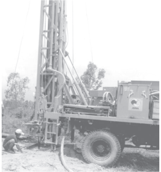
A drilling machine at work to sink a tubewell in Muse, Shan State (North). PBANRDA
