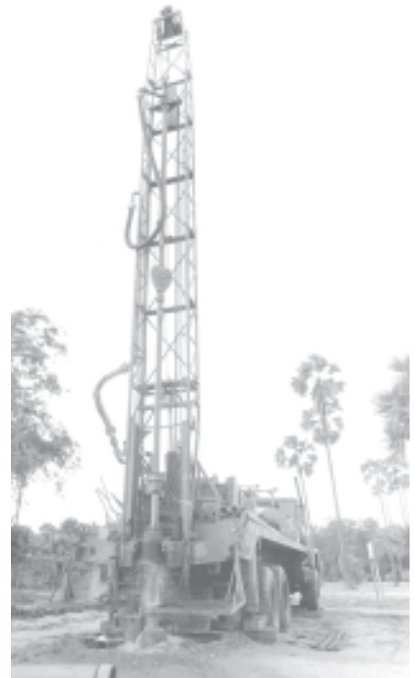
A tube-well sinking truck in action in Pyibin Village, Chauk Township, Magway Division, to supply potable water to rural people. — PBANRDA
