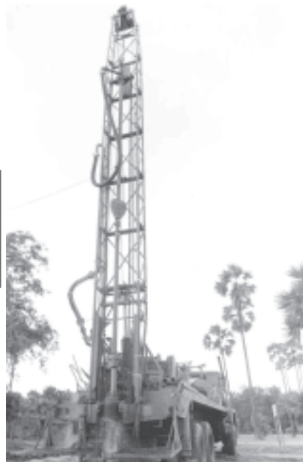
A tube-well sinking truck in action in Pyibin Village, Chauk Township, Magway Division to supply potable water to rural people.
